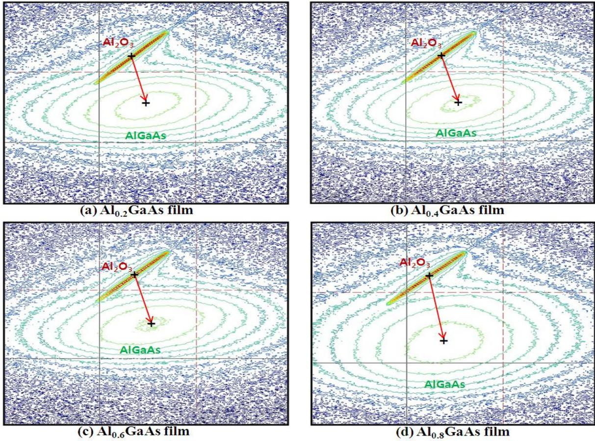
Fig. 5. XRD map images showing d-spacing between Al<sub>2</sub>O<sub>3</sub> and AlGaAs films having various Al compositions.
