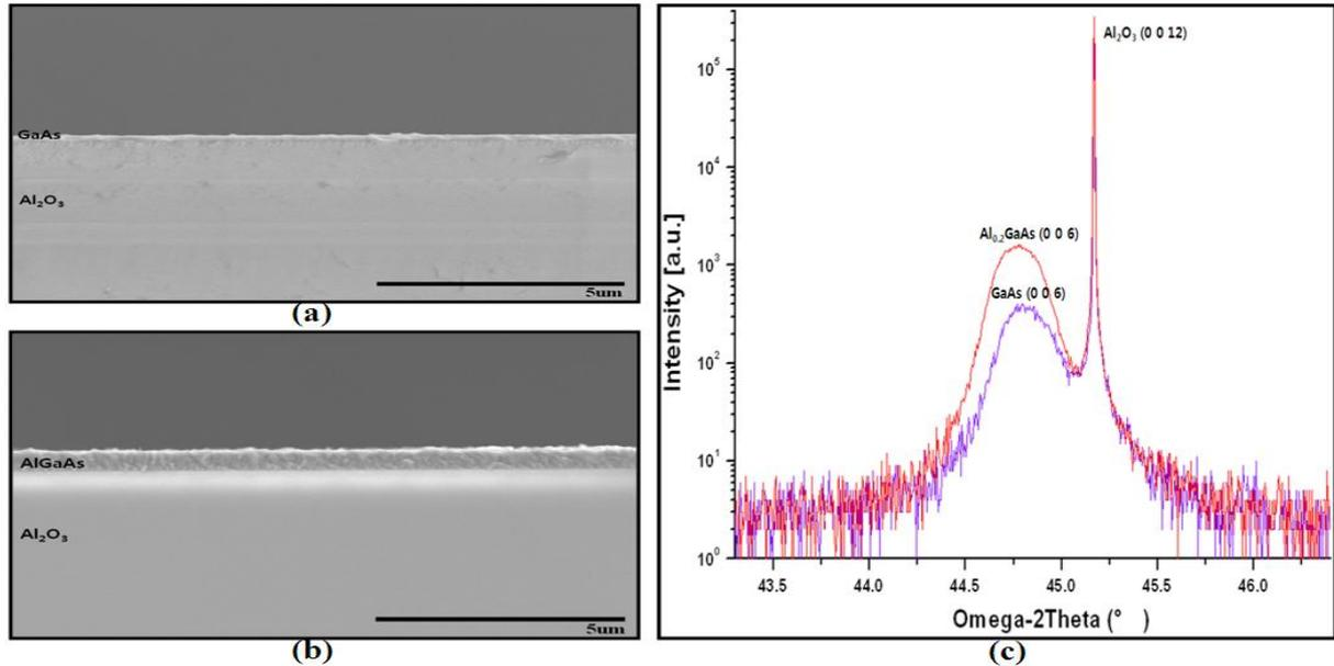
Fig. 1. (a)-(b) SEM and (c) XRD images for AlGaAs and GaAs films grown on Al<sub>2</sub>O<sub>3</sub> substrates.
