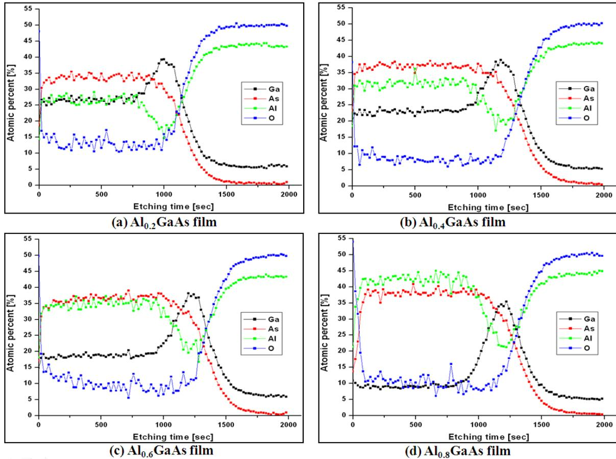
Fig. 3. XPS analyses of AlGaAs films having various Al compositions on an Al<sub>2</sub>O<sub>3</sub> substrate.
