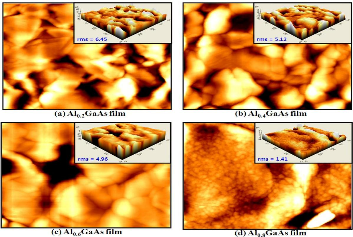
Fig. 4. AFM images for AlGaAs films having various Al compositions on an Al<sub>2</sub>O<sub>3</sub> substrate.
