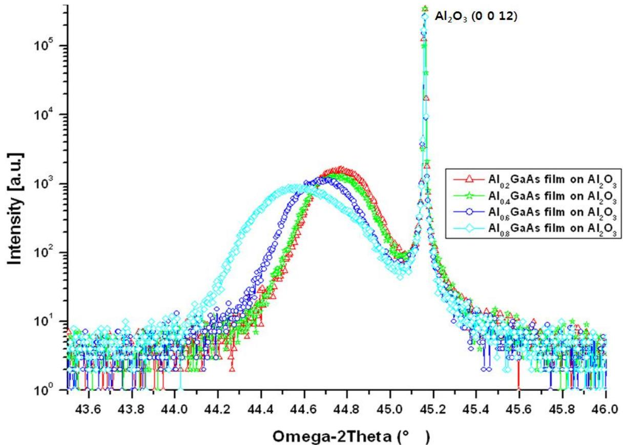
Fig. 2. XRD results for AlGaAs films having various Al compositions on an Al<sub>2</sub>O<sub>3</sub> substrate.
