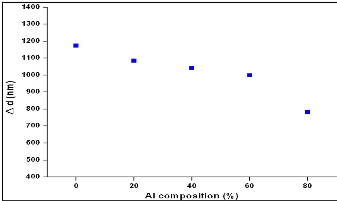
Fig. 6. Results of d-spacing obtained between Al<sub>2</sub>O<sub>3</sub> and AlGaAs films having various Al compositions.
